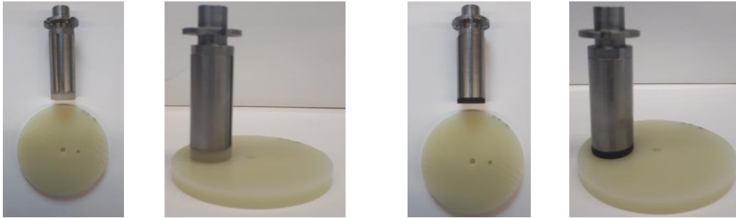
Figure 2. The polyamide plates in contact with the PA46 disk.
